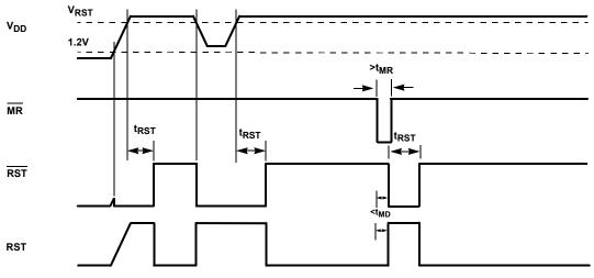
FIGURE 3. RST,  $\overline{\text{RST}}, \overline{\text{MR}}$  and  $\overline{\text{WDO}}$  timing diagram
