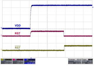
FIGURE 9. ISL706xRH RESET AND RESET ASSERTION
