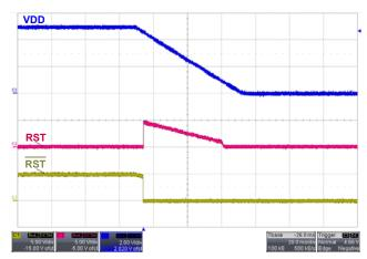
FIGURE 10. ISL705xRH RESET AND RESET DEASSERTION
